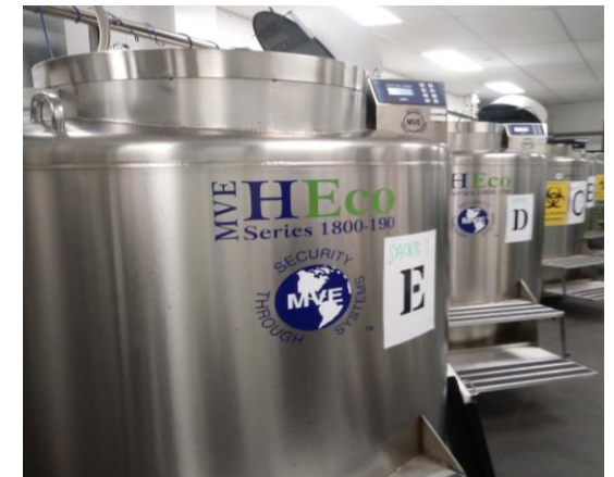
Cryogenic tanks storing SACRB biospecimens
