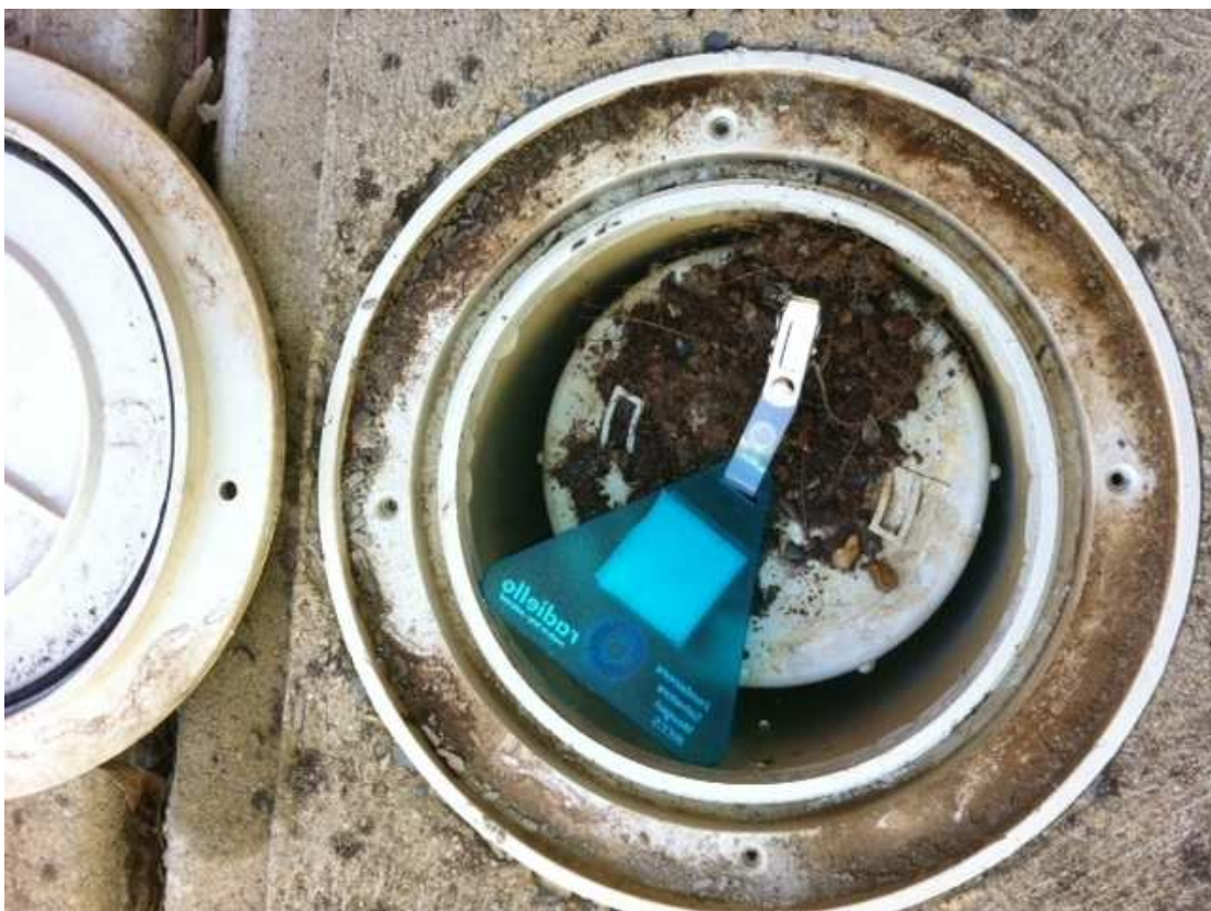
Figure 11: Monitoring volatile chlorinated compounds in a domestic service conduit at Clovelly Park using a Radiello® diffuse gas sampler.
